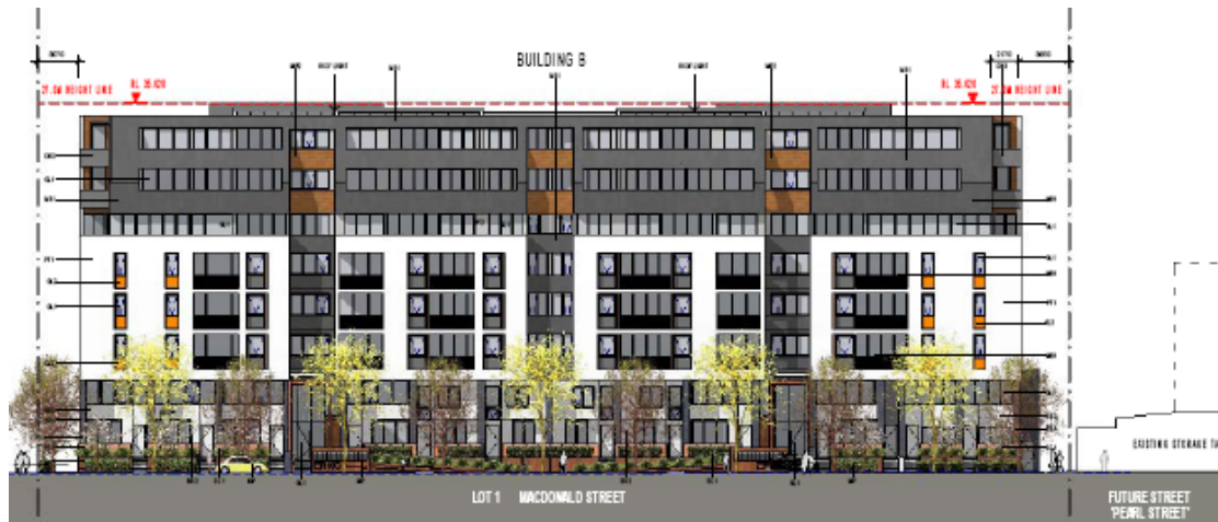
Figure 27: Building B elevation showing proposed facade modulation to MacDonal Street – Amended scheme
